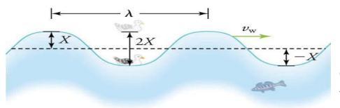
Consider the periodic water wave in Figure. Its wavelength is the distance
