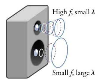
Because they travel at the same speed in a given medium, low-frequency sounds must have a greater wavelength than high-frequency sounds. Here, the lower-frequency sounds are emitted by the large speaker, called a woofer, while the higher-frequency sounds are emitted by the small speaker, called a tweeter.
